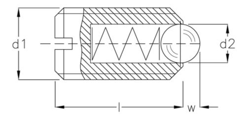
$\begin{array}{ll} \text{d1} & = \text{M8} \\ \text{d2} & = 5.0 \\ \text{I} & = 16 \\ \text{Spring pressure N bottom} = 35 \\ \text{Spring pressure N top} & = 20 \\ \text{W} & = 1.5 \\ \end{array}$
